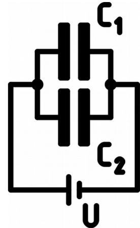
$$C = C_1 + C_2 + \dots$$
